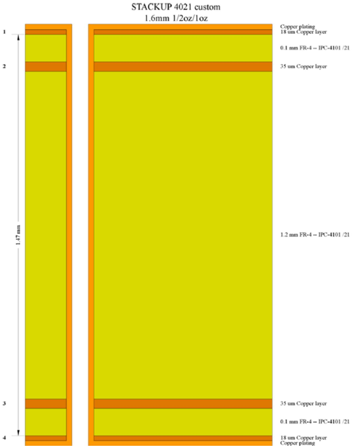
Figure 11: nRF9160 reference PCB (Elprint's 4-layer 4001 stack-up)
