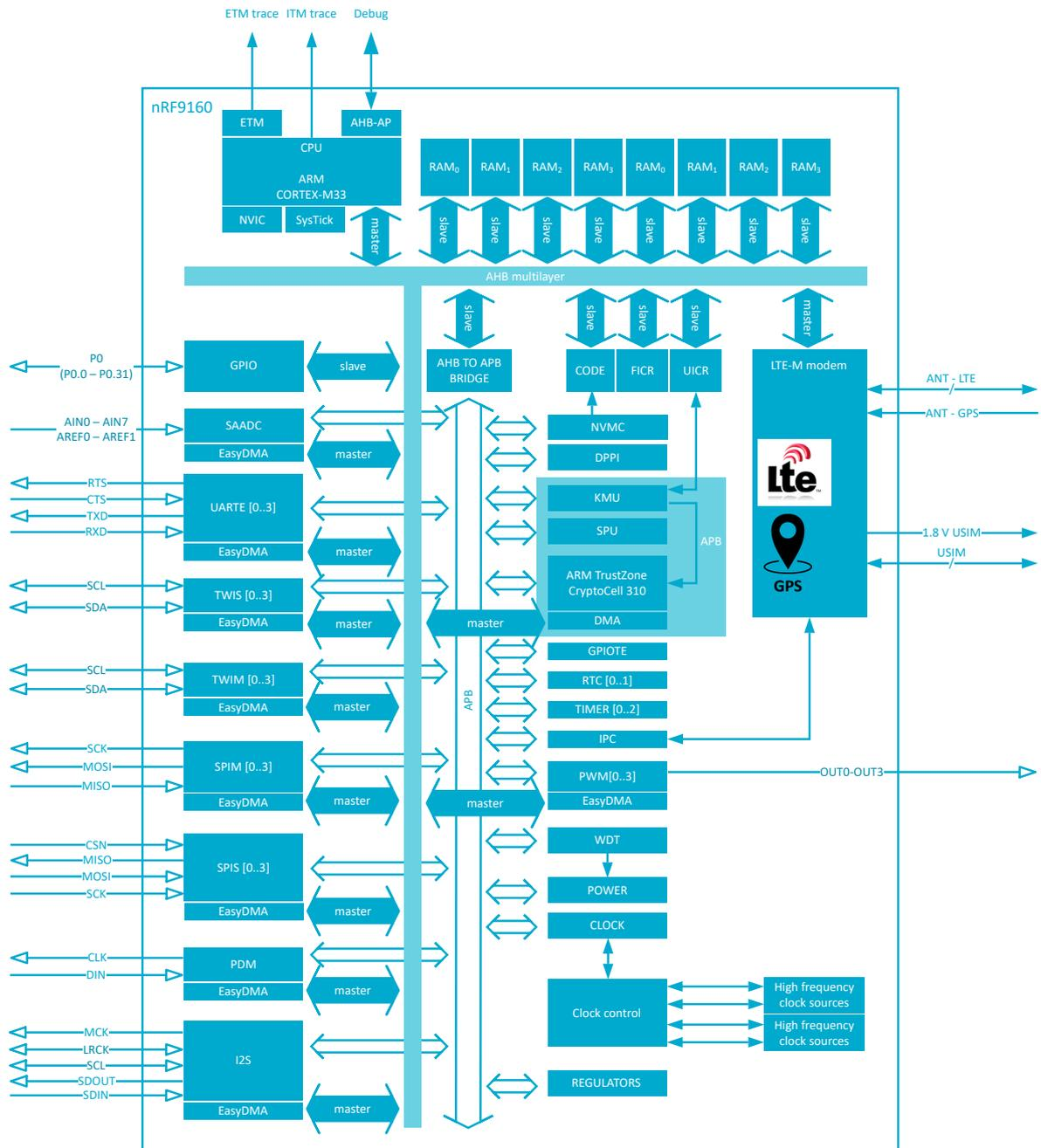
Figure 1: nRF9160 module block diagram
