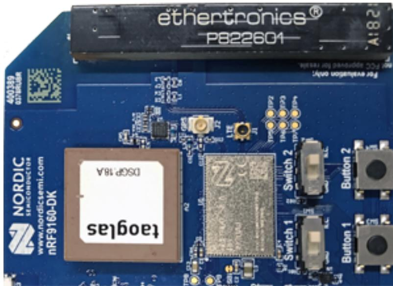
Figure 12: nRF9160 Development Kit antenna
