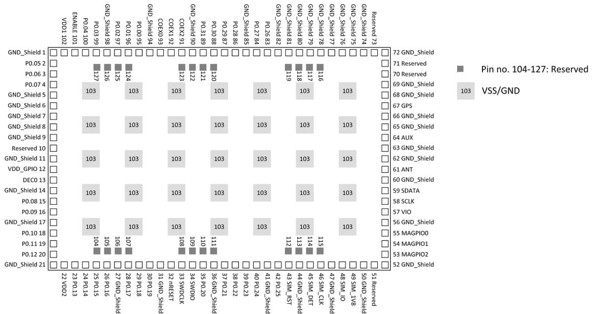
Figure 2: nRF9160 pinout, top (seen through module)
