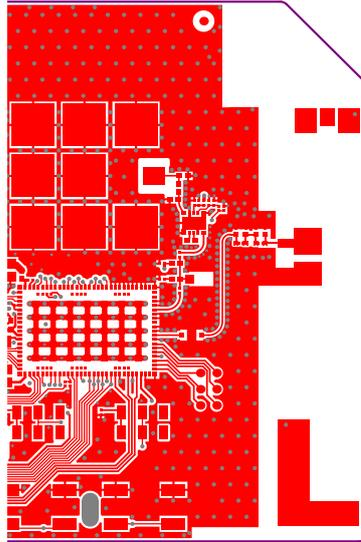
Figure 9: nRF9160 reference layout, metal layer 1 (top)
